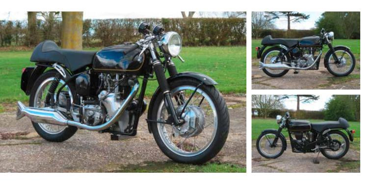
Introduced in 1956, the Venom sports roadster was derived from the touring MSS. The latter had disappeared from the range in 1948, reappearing in 1954 with a new swinging-arm frame and telescopic fork. The engine too was up-dated, changing to 'square' bore and stroke dimensions of 86x86mm and gaining an alloy cylinder barrel and 'head. Engine development pursued as part of the scrambles programme bore fruit in 1956 in the shape of the high-performance Venom and its 350cc sibling, the Viper.
