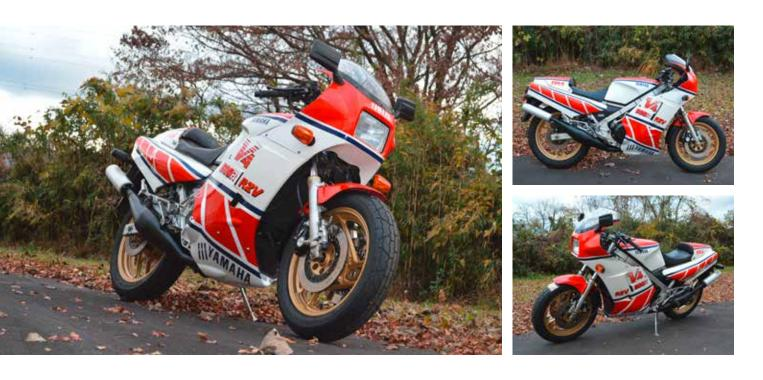
'Before 1983 Joe Public could only imagine what top-class racing equipment might be like to ride. Then Yamaha revealed the RD500LC. Here was everything on the wish list: the water-cooled V4 engine sprouting a multipack of expansion chambers, a mirror of the twin-crank V4s campaigned by Kenny Roberts. Its screaming 88bhp motor powered a lithe 392-pound package wearing all the factory racing graphics...' -Classic & Motorcycle Mechanics.
