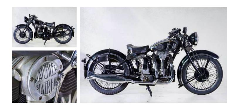
Reviewing the v-four Silver Hawk at its launch in the autumn of 1930, Motor Cycling stated that this exciting overhead-camshaft model was 'designed primarily to give really high speed, and to give this speed with silence and the added safety of a spring frame'.
