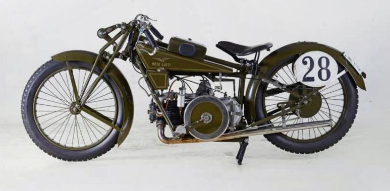
Weighing 290lbs and producing 8bhp, the Normale was good for around 50mph flat out. Although not intended for competition, the Normale was raced by the works prior to the arrival of the purposebuilt Corsa 2V for 1923, winning the prestigious Targa Florio endurance classic in 1922. A Tipo Sport spin-off with more powerful engine was catalogued for the first time the following year.
